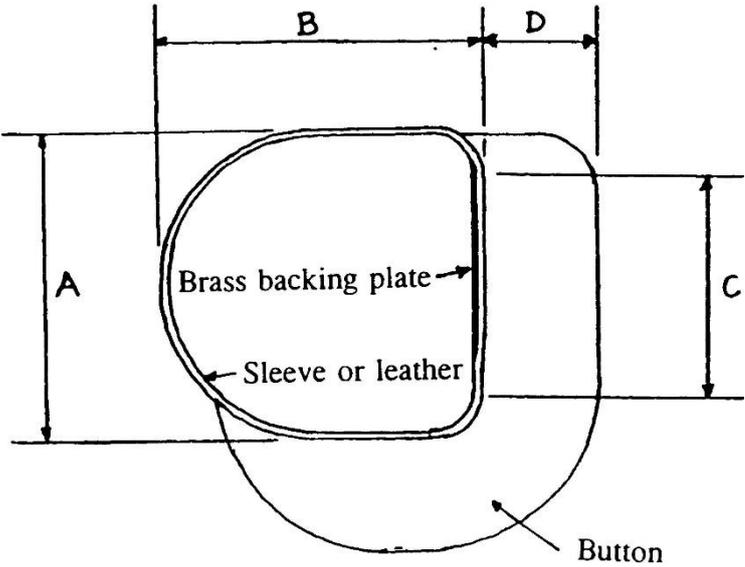
Figure 6 - VIEW OF SCULL CROSS SECTION FROM 'a-a'
